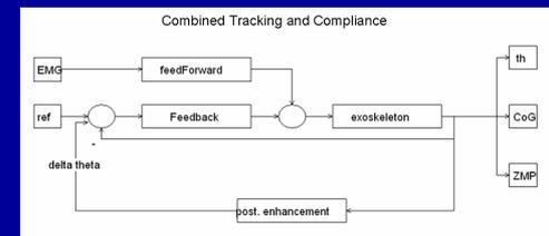
Fig 2. Combined 1) tracking and compliance control from theta and EMG (inner loop) and 2) postural equilibrium enhancement through ZMP measure and COG calculation (outer loop).
